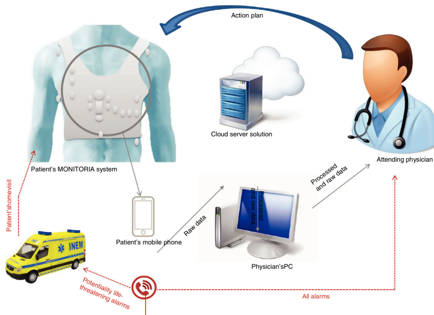
Figure 3 Generic representation of MONITORIA’s remote monitoring system.
