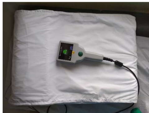
Figure 1 Patient and hospital electronic system including the electronic unit, antenna, and pillow.
